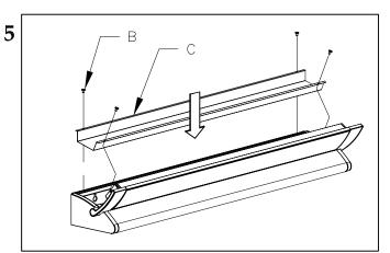
REINSTALL THE WIREWAY COVER<C> AND FASTEN THE SCREWS<B>.
