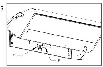
REINSTALL ACCESS PLATE<E> AND LOWER THE LUMINAIRE. MAKE SURE THE WIRE BUNDLE WITH FIBERGLASS SLEEVE<F> IS INSIDE LUMINAIRE AND NOT PINCHED BETWEEN HOUSING AND WALL PLATE
