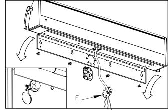
SWING OPEN HINGED MOUNTING PLATE. REMOVE ACCESS PLATE<E> FROM MOUNTING PLATE. INSTALL LUMINAIRE BY HOOKING ONTO FOUR SCREWS ON THE WALL THROUGH KEYHOLE SLOTS ON MOUNTING PLATE.
