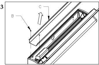
SWING EXAM LIGHT SECTION FORWARD, UNSCREW FOUR #8 SCREWS<B> AND REMOVE WIREWAY COVER<C> TO EXPOSE WIRING COMPARTMENT.
