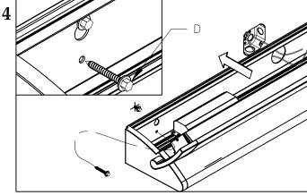
INSTALL LUMINAIRE BY HOOKING ONTO TWO SCREWS ON THE WALL (BY OTHERS) THROUGH KEYHOLE SLOTS OF LUMINARE (SEE INSET). TIGHTEN MOUNTING SCREWS AGAINST HOUSING AS SHOWN IN INSET. INSTALL TWO BOTTOM  $\frac{1}{4}"$  DIAMETER SCREWS<D> (BY OTHERS) TO LUMINAIRE. MAKE ELECTRICAL CONNECTIONS.
