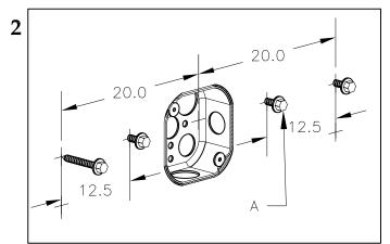
INSTALL FOUR UPPER MOUNTING SCREWS<A>(SUPPLIED BY OTHERS). 1/4 " DIAMETER SCREWS WITH WASHER HEAD ARE RECOMENDED (.70" MAXIMUM WASHER DIAMETER). LEAVE ABOUT 1/4" SPACING BETWEEN SURFACE AND WASHER.
