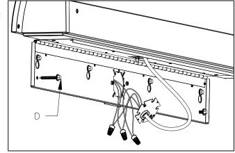
TIGHTEN MOUNTING SCREWS AGAINST MOUNTING PLATE. INSTALL TWO  $\frac{1}{4}$ " DIAMETER BOTTOM SCREWS (BY OTHERS). MAKE ELECTRICAL CONNECTIONS.
