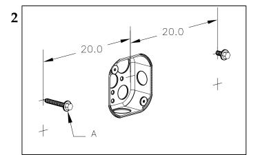
INSTALL TWO UPPER MOUNTING SCREWS <A> (SUPPLIED BY OTHERS). 1/4 " DIAMETER SCREWS WITH WASHER HEAD ARE RECOMENDED (.70" MAXIMUM WASHER DIAMETER). LEAVE ABOUT 1/4" SPACING BETWEEN SURFACE AND WASHER.
