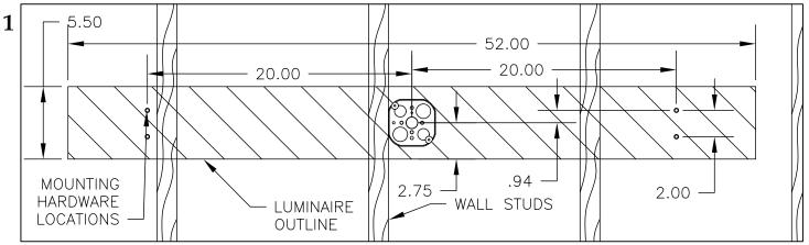
PREPARE LUMINAIRE MOUNTING AREA. THE HATCHED AREA SHOWN ABOVE TO BE REINFORCED TO SUPPORT LUMINAIRE. VERTICAL LOCATION OF CENTER OF JUNCTION BOX TO BE 2.75" ABOVE THE BOTTOM OF LUMINAIRE. MARK MOUNTING HOLE LOCATIONS PER DIMENSIONS SHOWN.
